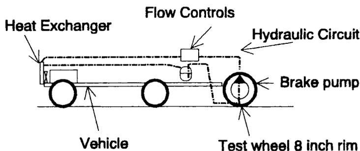
FIG. 2 Sample Brake Systems
