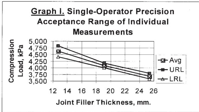
FIG. X3.1 Single-Operator Precision Acceptance Range of Individual Measurements
