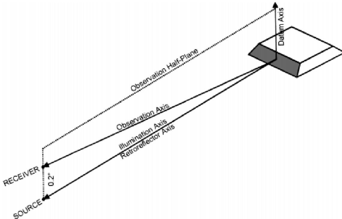
FIG. 2 Position of Marker for Photometry, 0° Entrance Angle
