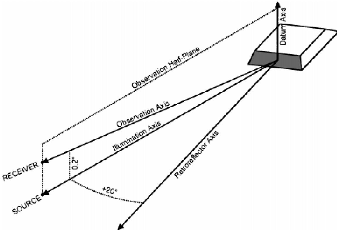
FIG. 3 Position of Marker for Photometry, +20° Entrance Angle
